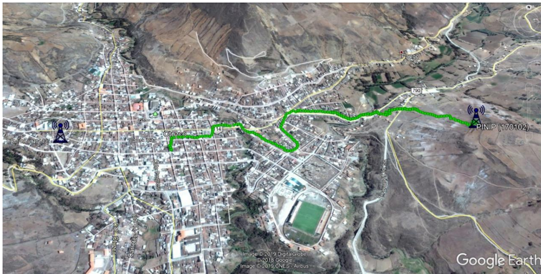
Figura 3.10. Recorrido Drive Test, eNodeB-Pinip-Otuzco
