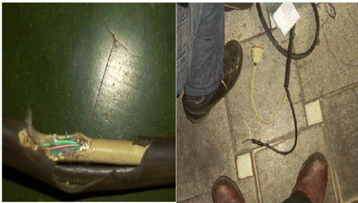
Figura 3.13: Cable data Power 12V
