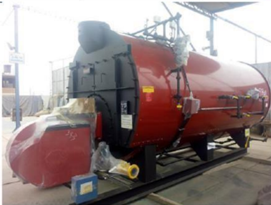
CALDERO HURST 500 BHP
