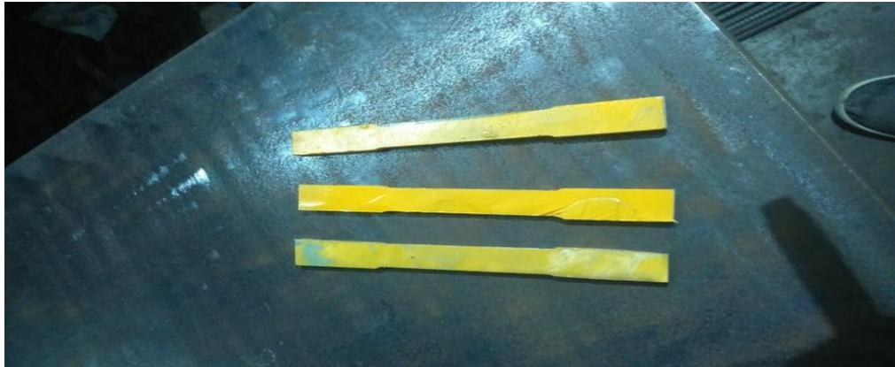
Figura 4: Probetas tipo dogbone - ASTM D638.
