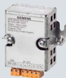
The Safe Brake Relay allows the Power Module to be safely connected to an electromechanical motor brake, allowing the brake to be directly and safely controlled by the Control Unit in accordance with EN 954-1 Safety Category 3 and IEC 61508 SIL 2.
