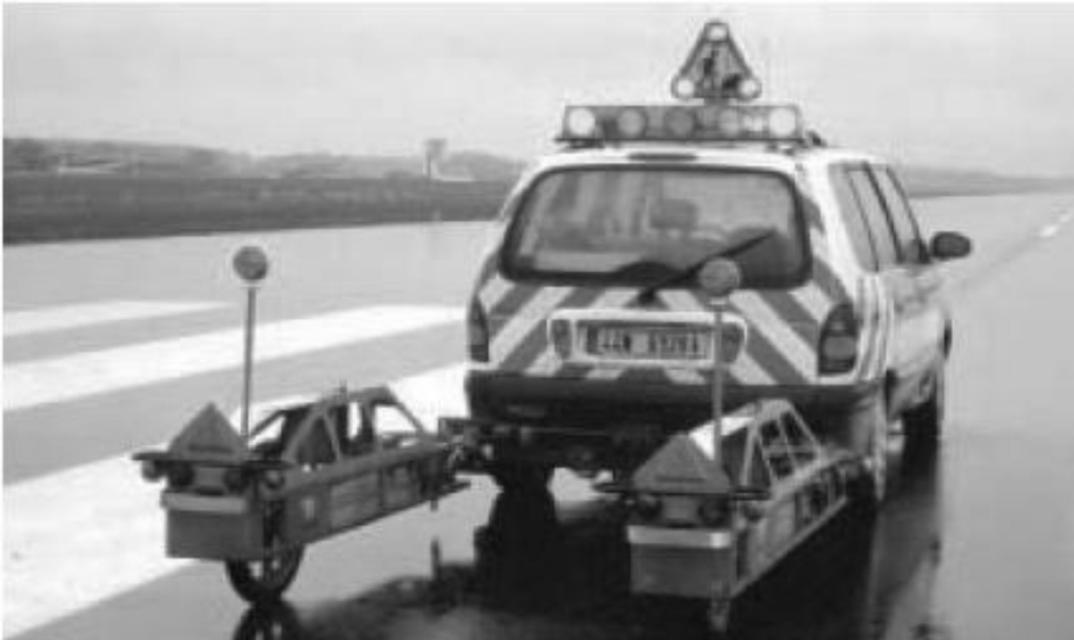
Fuente : University of South Florida Development and evaluation of an inertial based pavement roughness measuring system
