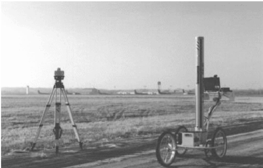
Fuente: University of South Florida Development and evaluation of an inertial based pavement roughness measuring system
