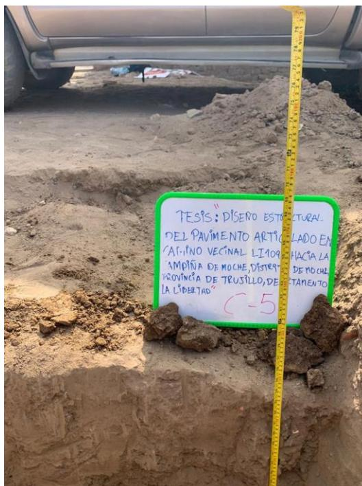
**Figura 14***Excavación Calicata 06*
