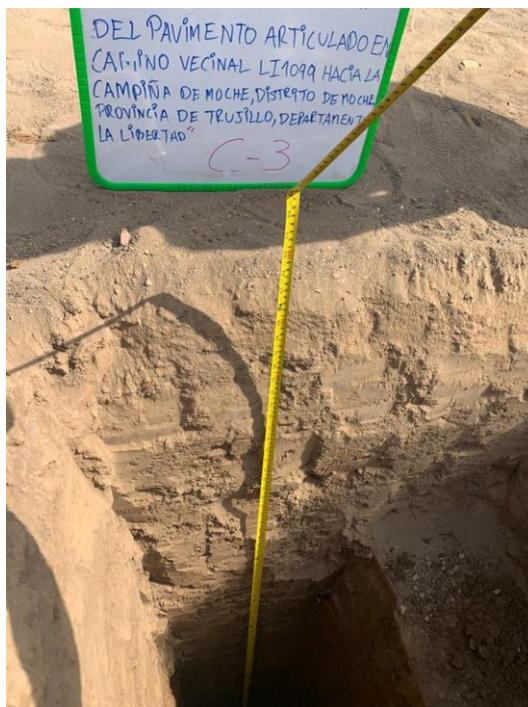
**Figura 12***Excavación Calicata 04*
