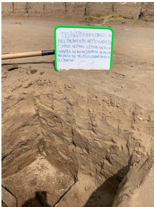
**Figura 10***Excavación Calicata 02*
