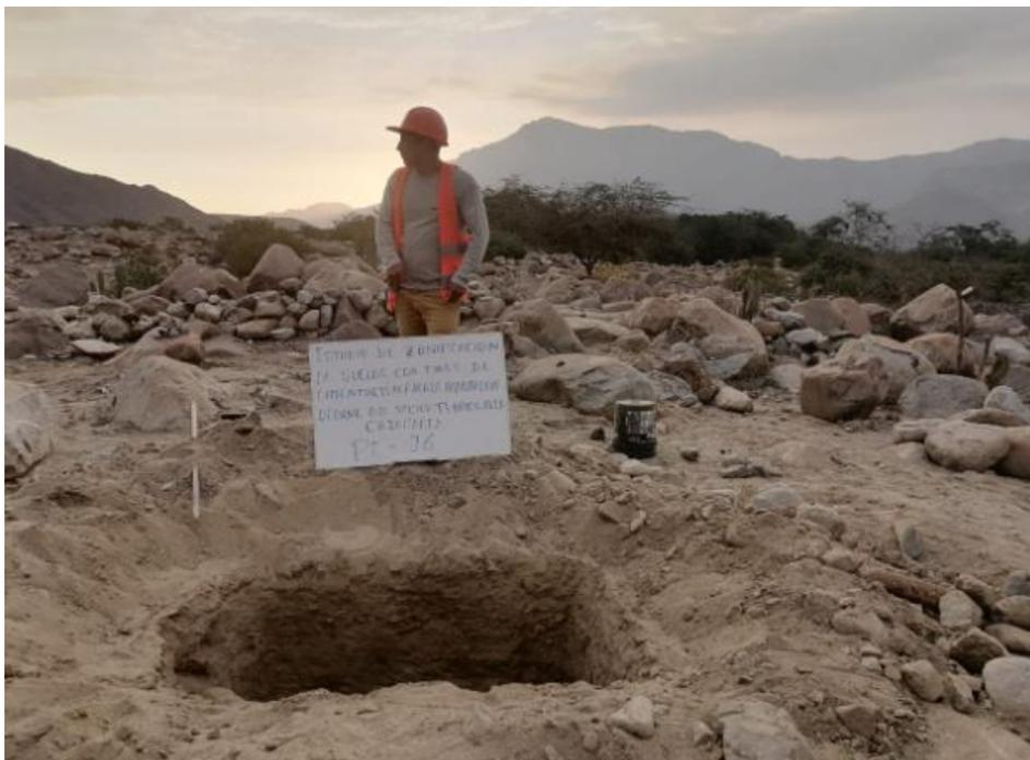
**Fotografía 08***Excavación de calicata C-07*
