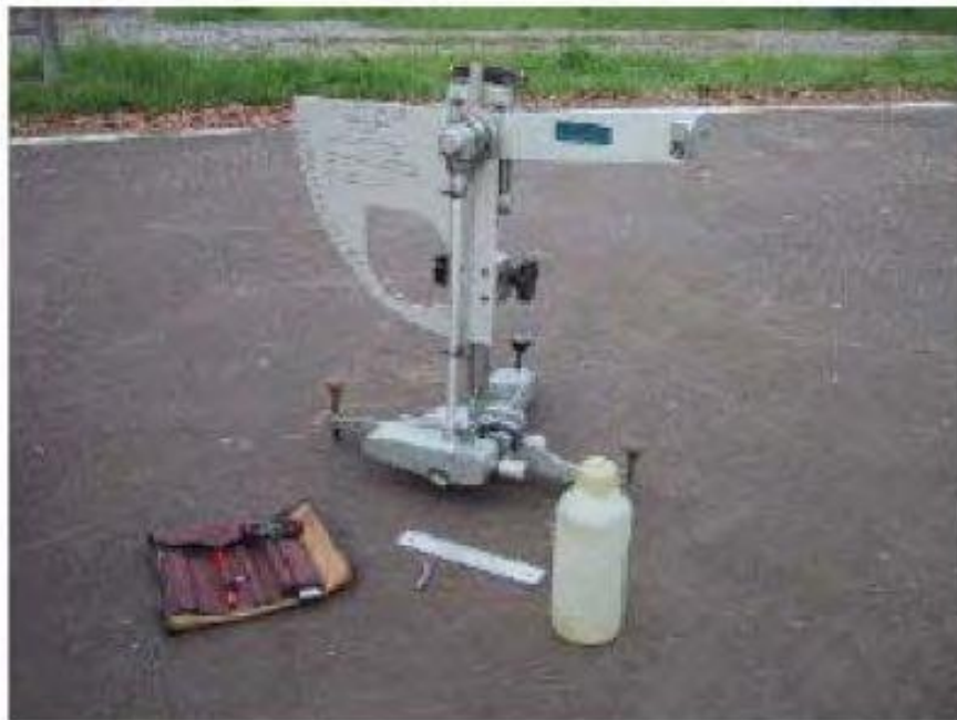
Figura N° 24 : Péndulo del TRRL (Transport and Road Research Laboratory)
